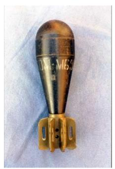
Nomenclature: U.S. Projectile, 60.00 mm, Mortar, Drill, M69
