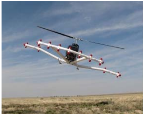
A helicopter like this is flying the old army depot site south of Edgemont, taking magnetic readings to determine possible contamination sites. Photo courtesy of Battelle Institute
